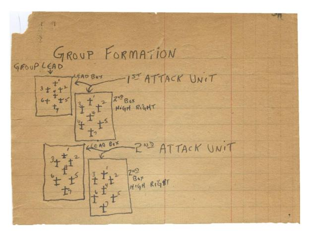
The group assembles thusly after take-off. Squadrons alternate with each mission, different box positions. Each squadron flies seven ships to form one box. Combat crews alternate ship positions within their respective squadron boxes.
