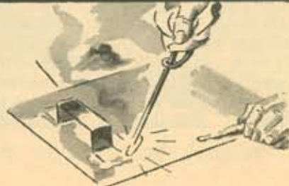
SOLDERING. Specks of solder salvaged from can tops were applied with rods from the handles of jam buckets.
