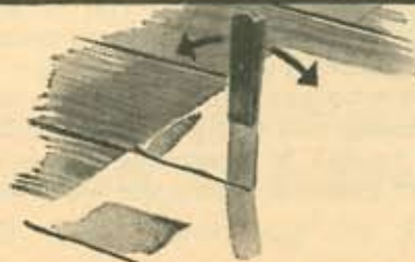
CUTTING of tin was managed with a knife blade stuck into a floor crack and worked to and fro like a can opener.
